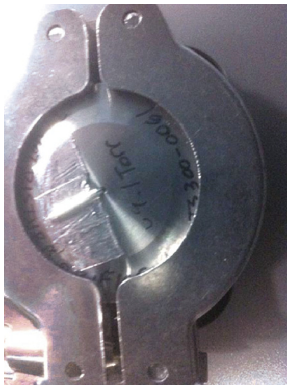
Figure 4 - Mechanical Leak (4.1 Torr shown)
